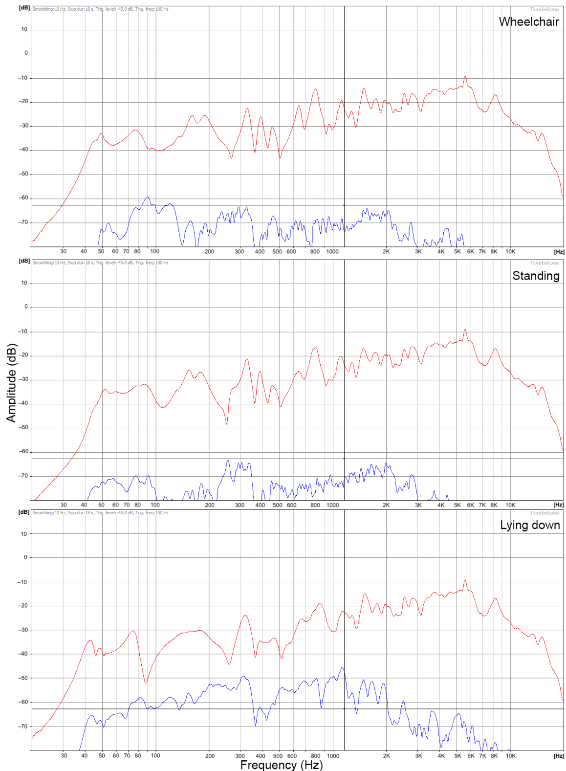
Figure 7. Results from accelerometer measurements on one of the small platforms in Sound Forest, with a researcher sitting in a wheelchair placed on the platform ( top ), standing on the platform ( middle ), and lying down on the platform ( bottom ). The red curve corresponds to audio captured using a microphone placed next to the ear. The blue curve corresponds to the signal recorded by the accelerometer.
