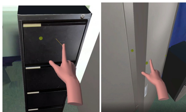
Figure 11. The left image shows the last point added to define a perpendicular behavior in AR. The right image shows in yellow the points to enable the rotation of the cabinet door in VR.
