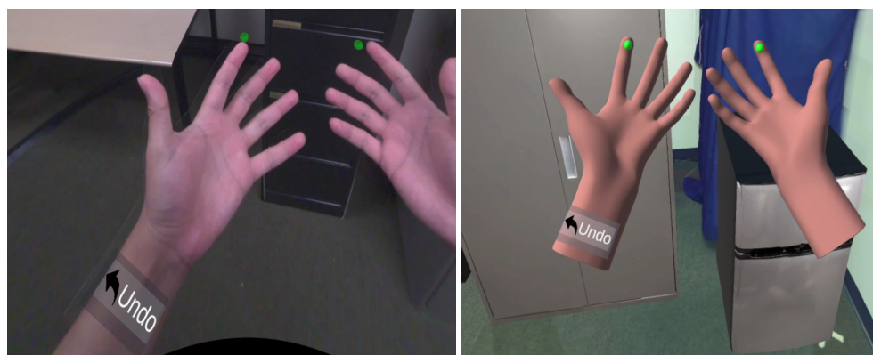
Figure 2. (Left) Hands visualized in AR. (Right) Virtual hands in VR. Green spheres are pointers to interact with elements in the scene.
