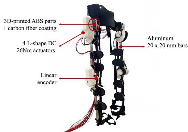
**Figure 2.** ALICE lower-limb exoskeleton. The picture represents the open-source, active lower-limb exoskeleton employed in the protocol and available at the IAS-LAB of Padova University.
