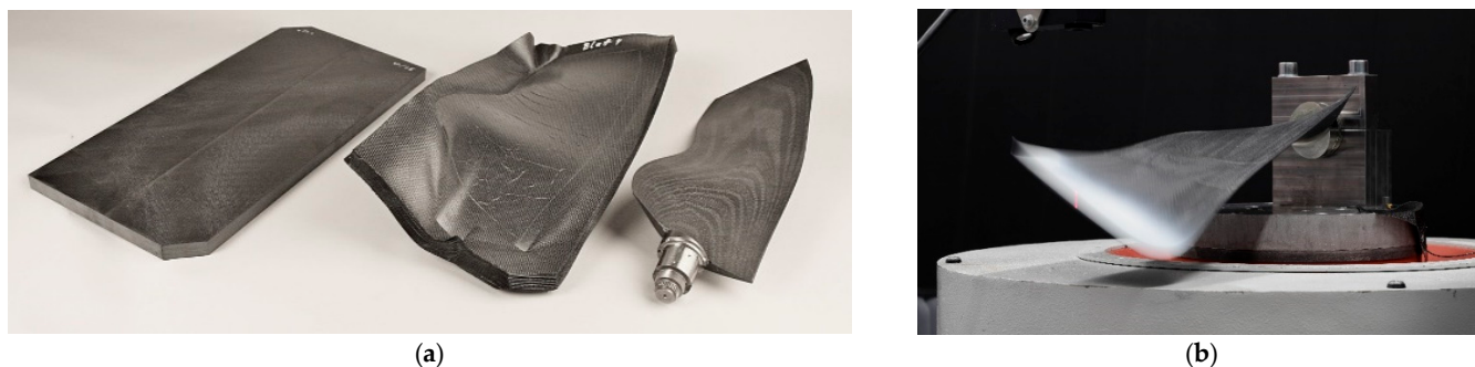
Figure 2. Manufacturing process of the CFRP blades (a) and the shaker test (b) [5].
