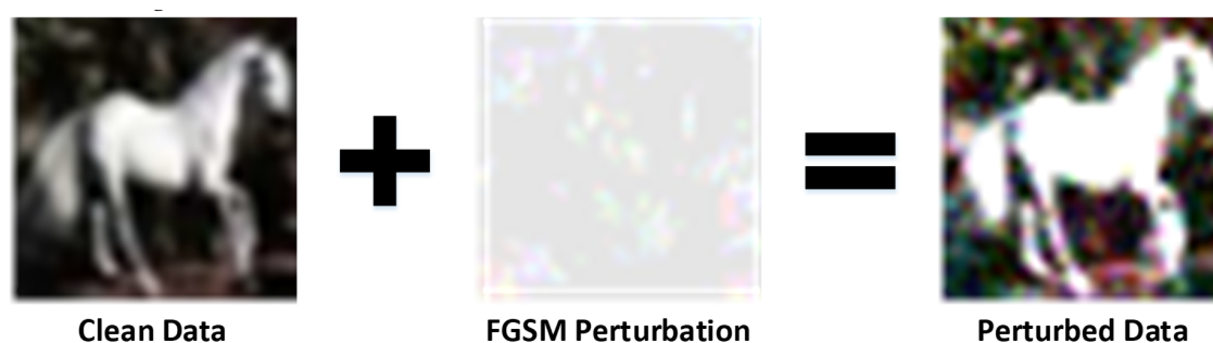
Figure 1. The figure shows injecting a perturbation from the Fast Gradient Sign Method (FGSM) attack into a sample image from the ten-class Canadian Institute for Advanced Research (CIFAR) dataset. A high amount of perturbation is chosen during the simulation for better visual presentation.
