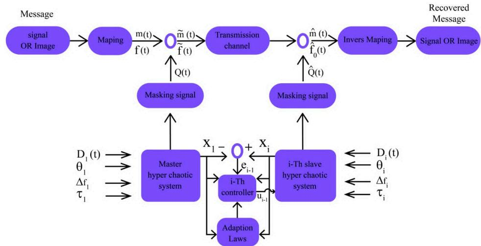
Figure 2. Block diagram of chaotic masking with multi-state synchronization for the distributed system.
