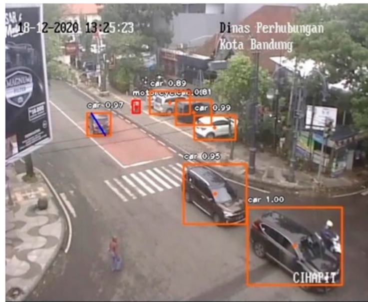
Figure 5. Detection result on the frame of CCTV stream.
