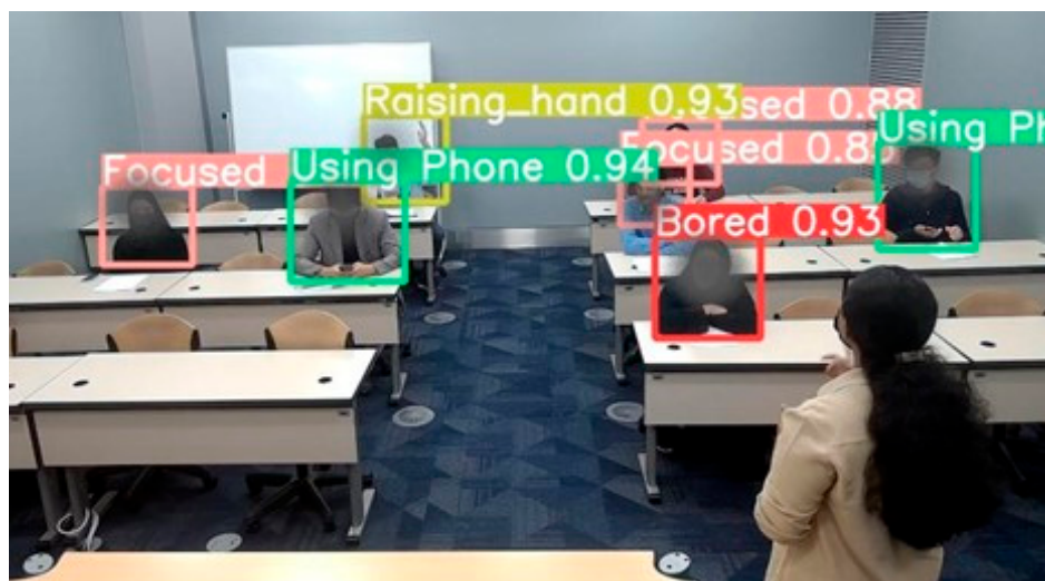
Figure 9. Classroom setup for experimentation on seven students. Each student's action is detected and color-coded. Three students are focused, two are using their phones, one is bored, and the other is raising his/her hand.
