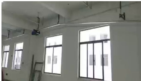
Simulated environment (indoor simulated tunnel environment, inspection robot track installation height: 5 m)
