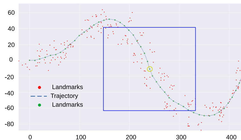
Figure 3. Slide window (square) associated with a robot pose (highlighted with a circle); RectangleSize = size(H) .
