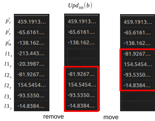
Figure 5. Simple example of updating matrix b where N_{lm} = 1 and k = 3 . The red box highlights the items that are moved during the update.
