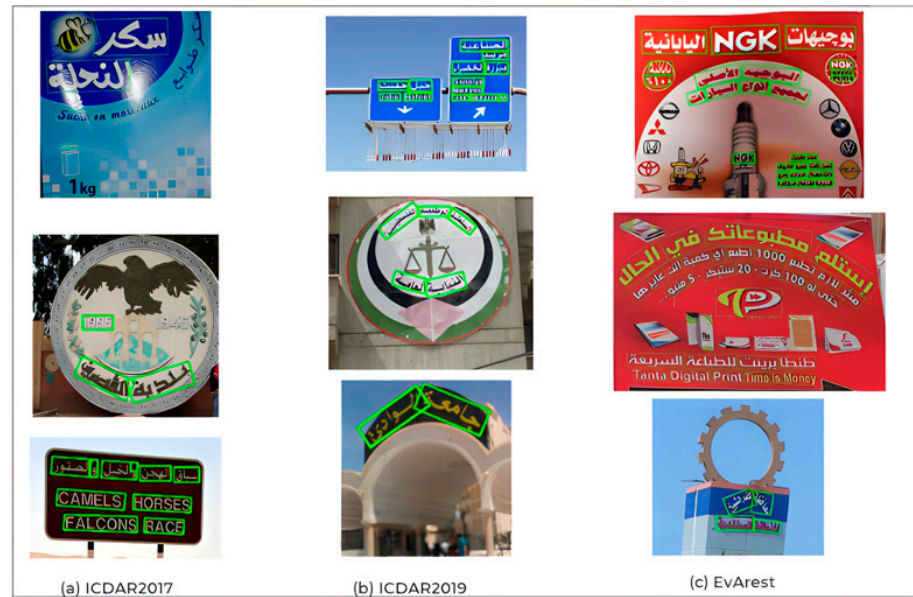
Figure 11. Qualitative text localization results of the model from: (a) ICDAR2017 [39]; (b) ICDAR2019 [41]; and (c) EvArest [10]. Green boxes refer to results of localization phase.
