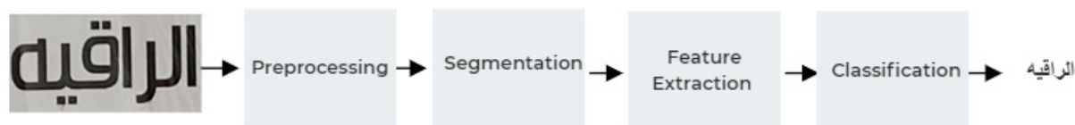
Figure 2. Phases of recognition text from natural scene images, image from the EvArEST dataset [10]. The word in image means “Elegant” in English terms.
