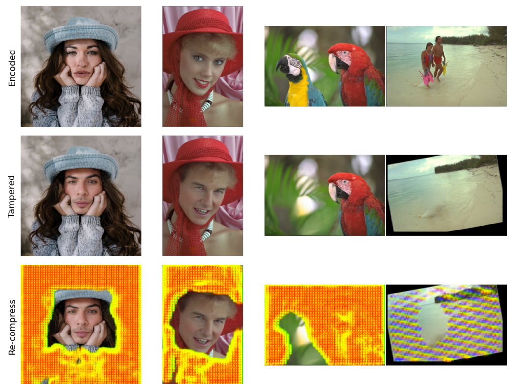
Figure 6. The results of the Balle2018 + \mathcal{P}_{LPIPS} SLIC images were re-compressed after GenAI manipulation: faceswap and stable diffusion inpainting.
