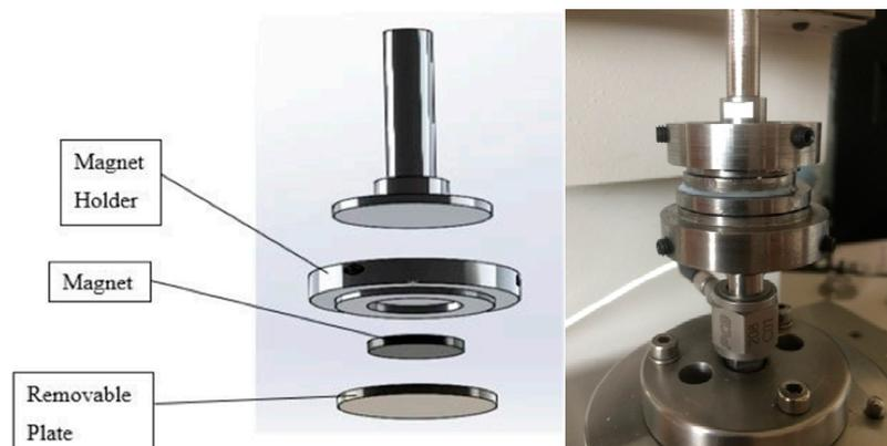
**Figure 8.** Design of top plate (left) and entire test assembly (right).
