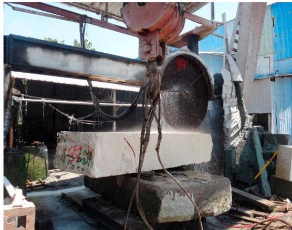
**Figure 4.** The block of natural marble rock was cut by a special saw.
