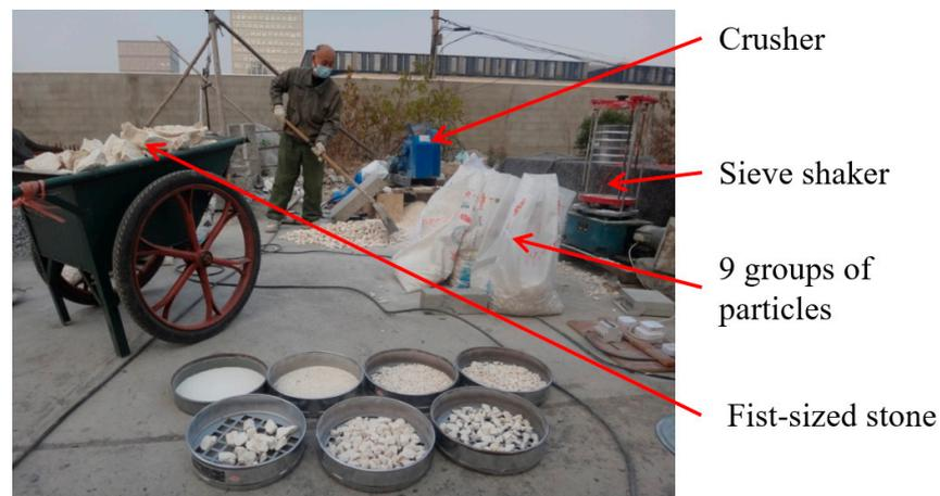
**Figure 5.** The process of marble particles being divided into 9 groups.
