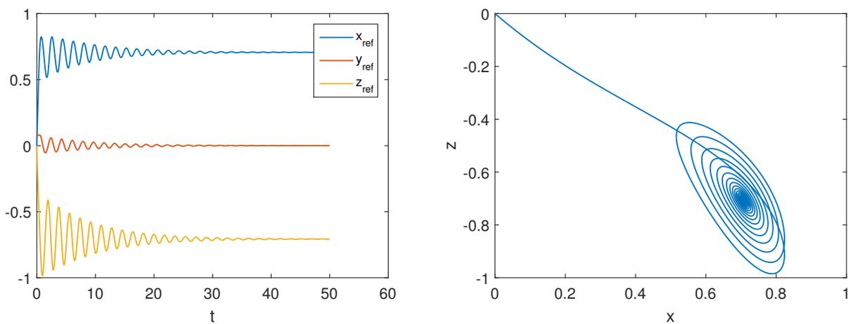
**Figure 2.** Chua’s circuit: (left)—solution plot; (right)—the curve  $(x_{ref}, z_{ref})$  in the  $(x, z)$  plane.
