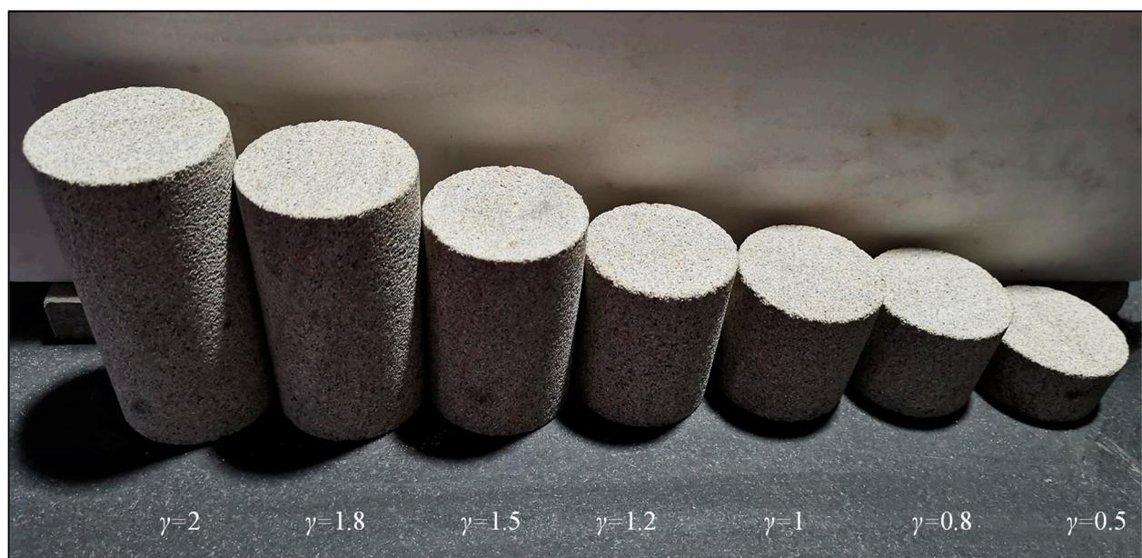
**Figure 4.** Samples of coal-bearing sandstone under different length–diameter ratios.
