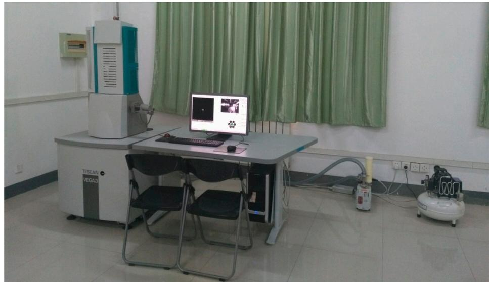
**Figure 3.** Scanning electron microscope system.
