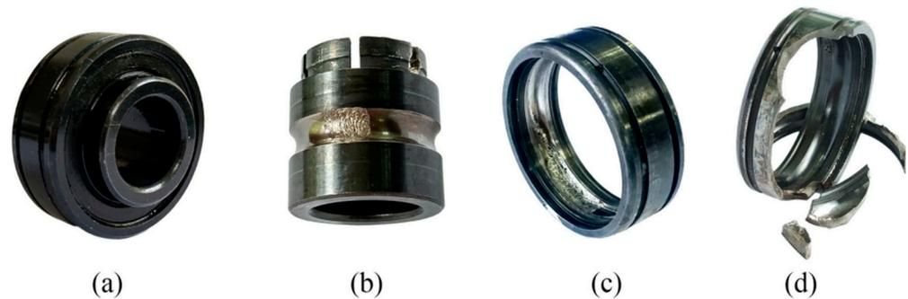
**Figure 4.** Photos of tested bearings: (a) normal bearing, (b) inner race wear, (c) outer race wear, and (d) outer race fracture.
