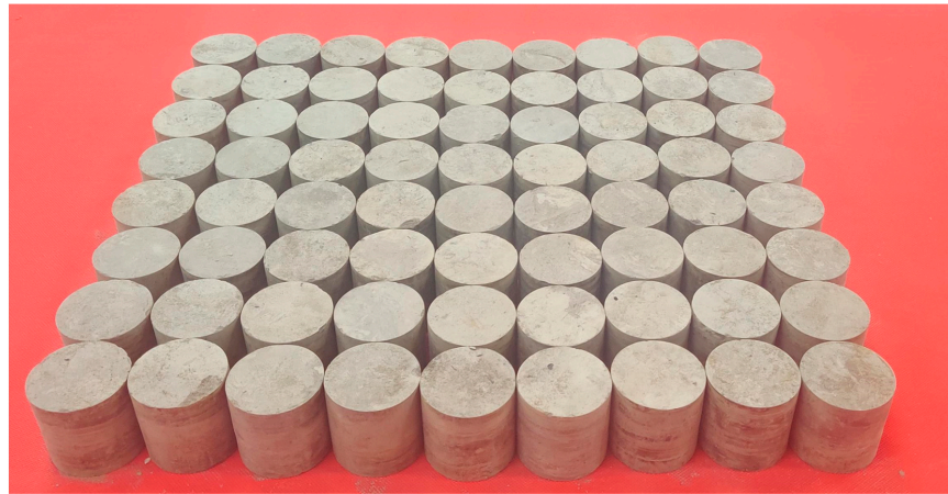
Figure 2. Coal-bearing mudstone specimens.
