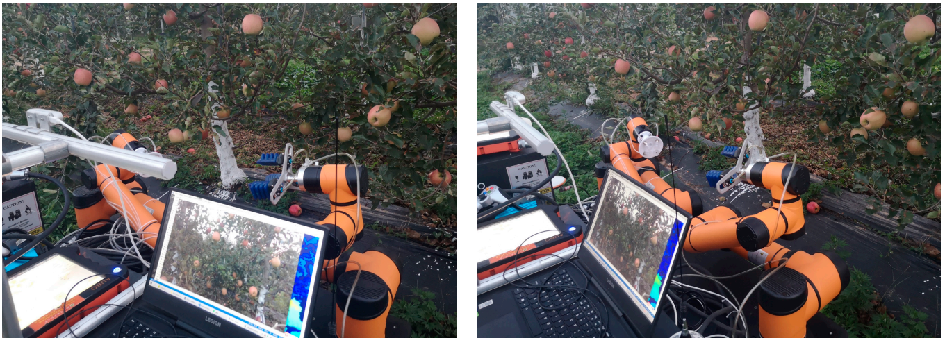
Figure 25. Verification situation of the test for estimating the maximum diameter of fruit on apple trees.
