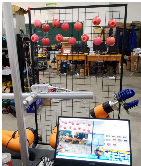
Figure 17. Validation test situations for maximum diameter estimation of imitation apples in the laboratory.
