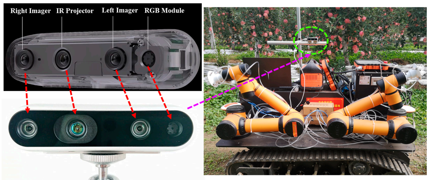
Figure 4. Module composition of the Intel Realsense D435 camera and its assembly on the apple-picking robot.
