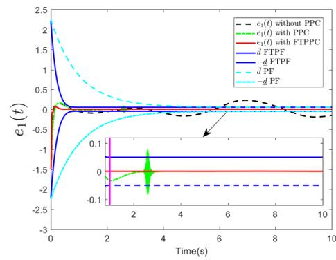
Figure 3. Error signals  $e_1(t)$  and performance functions  $\rho(t)$ .
