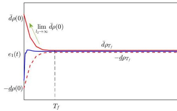
**Figure 1.** Performance functions  $\rho(t)$  and tracking error  $e_1(t)$ .
