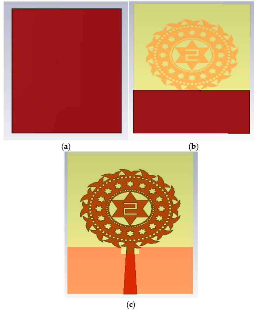
**Figure 6.** Various ground plane configurations: (a) FGPS (Full ground plane structure), (b) PGPS (Partial ground plane structure), (c) DPGS (Defected partial ground structure).
