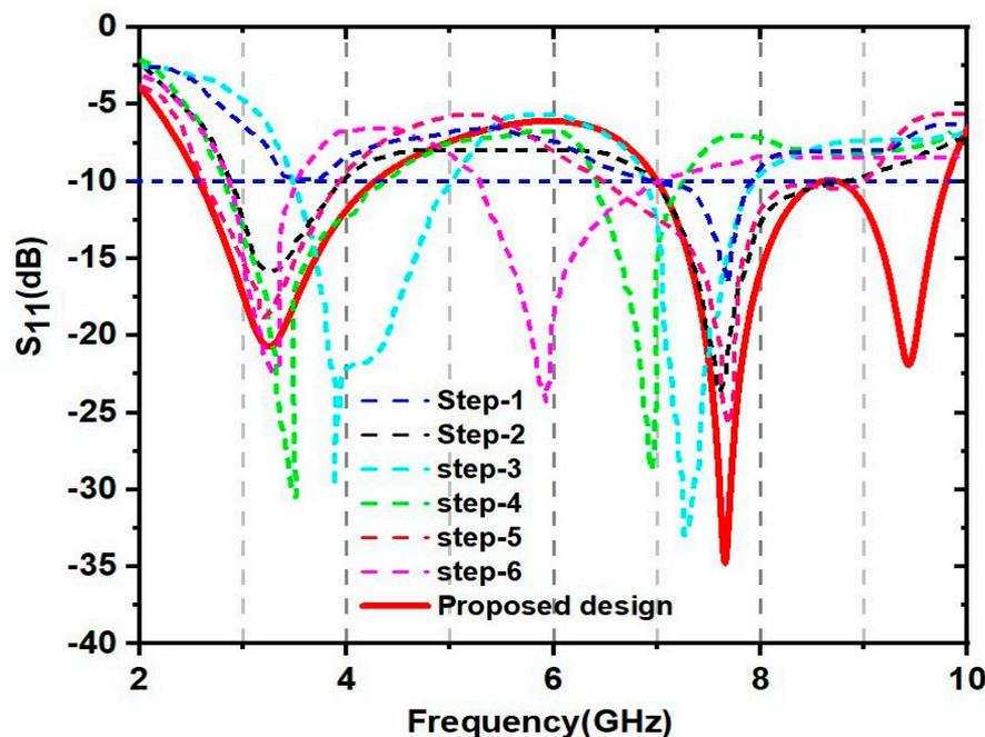
Figure 5.  $S_{11}$  (dB) values for each iteration step.
