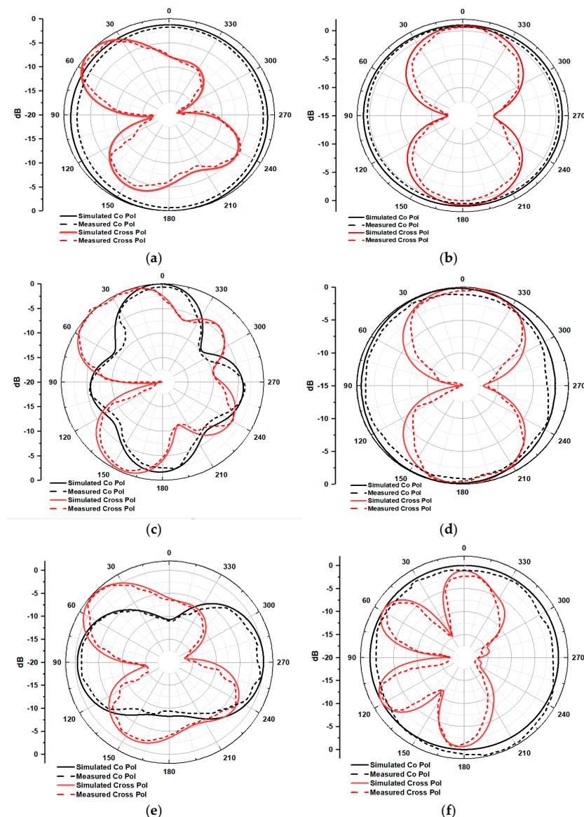
**Figure 18.** Co-pol and cross-pol radiation patterns: (a) 3.22 GHz E-Plane, (b) 3.22 GHz H-plane, (c) 7.64 GHz E-Plane, (d) 7.64 GHz H-Plane, (e) 9.41 GHz E-Plane, and (f) 9.41 GHz H-Plane.
