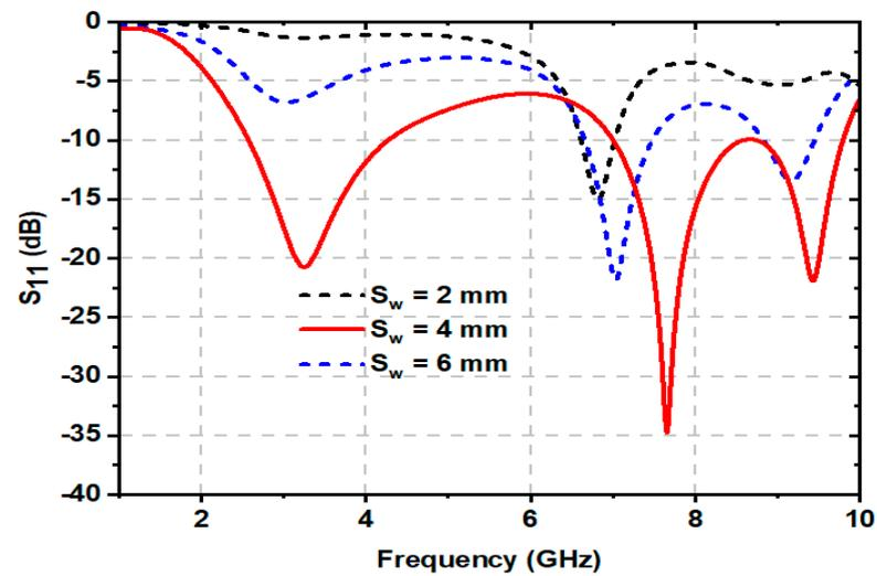
Figure 11. Simulated analysis of  $S_{11}$  (dB) response as a function of  $S_w$ .
