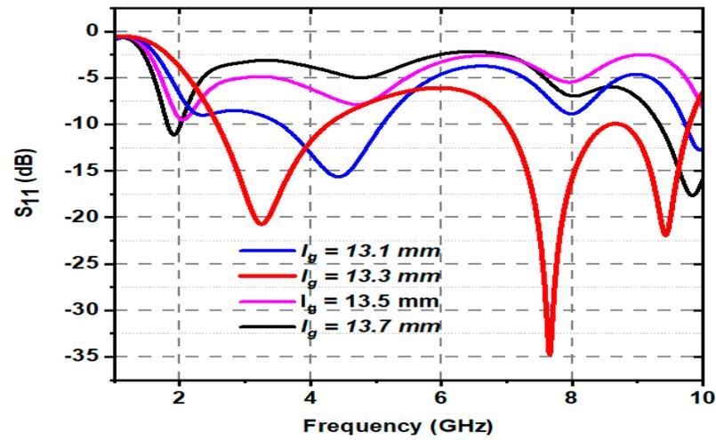
Figure 10. Simulated analysis of  $S_{11}$  (dB) response as a function of  $l_g$ .
