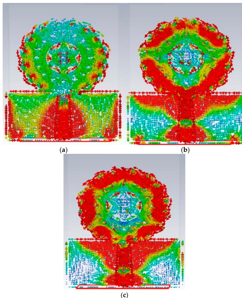
**Figure 21.** Plots of distributed Surface currents at resonating frequencies (a) 3.2 GHz (b) 7.6 GHz (c) 9.4 GHz.
