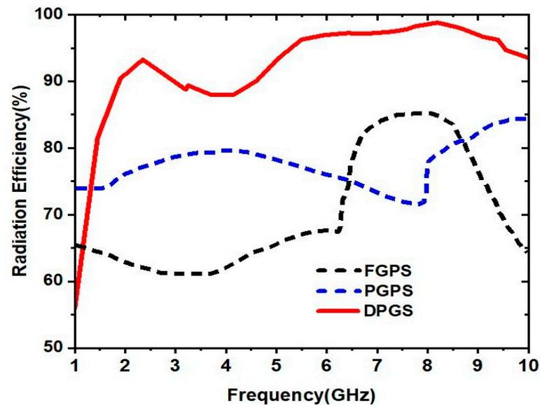
Figure 9. Variations in radiation efficiency for various ground plane structures.
