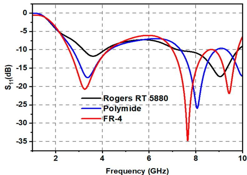
Figure 13.  $S_{11}$  (dB) response of the proposed antenna for different dielectric materials.
