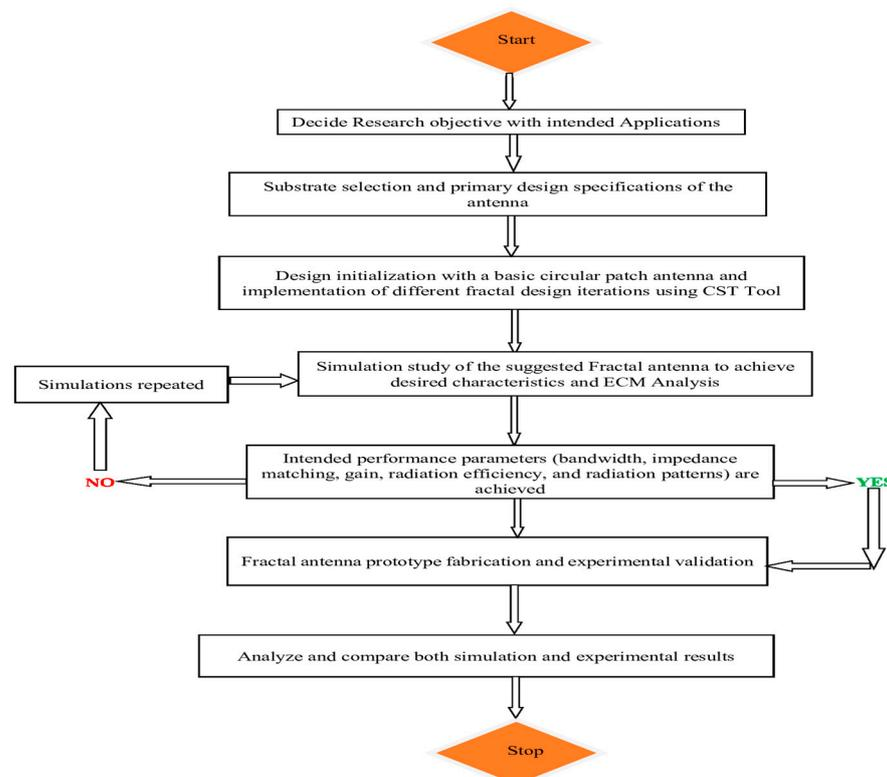
**Figure 1.** Design framework flowchart of the fractal antenna.
