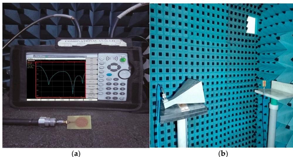
**Figure 15.** Images of the measuring setup of the proposed antenna: (a) VNA snapshot, (b) anechoic chamber with AUT.
