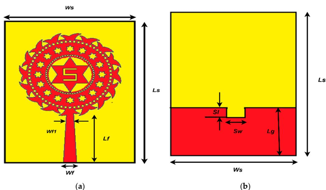
Figure 2. Proposed antenna: (a) front and (b) back views.
