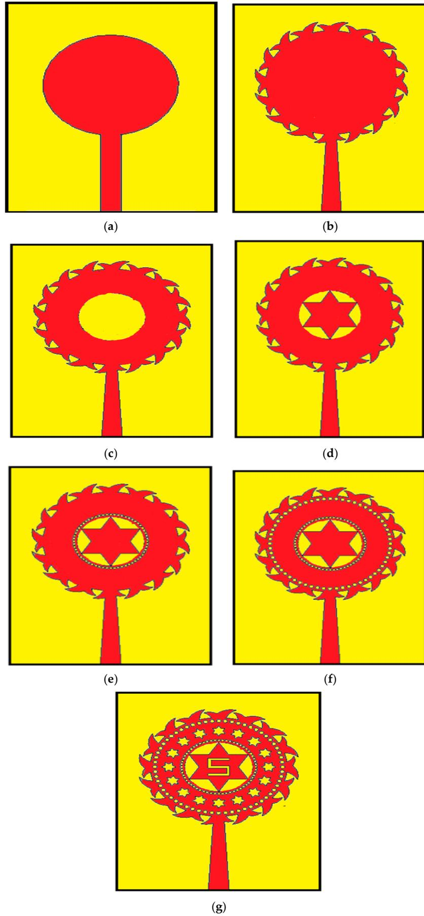
Figure 4. (a–g) Different iteration steps for designing the intended antenna.
