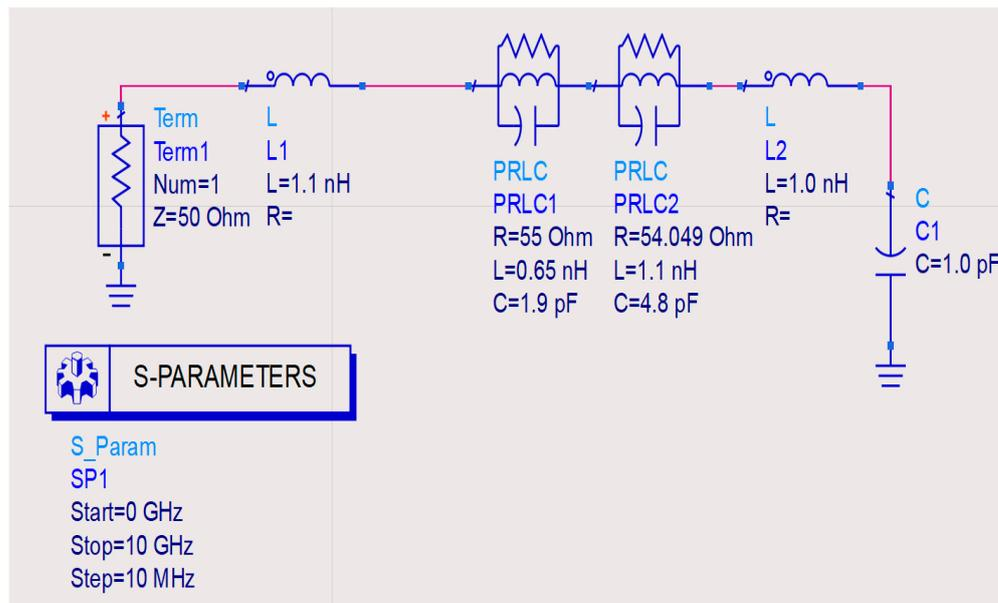
Figure 22. Equivalent circuit of the proposed antenna.
