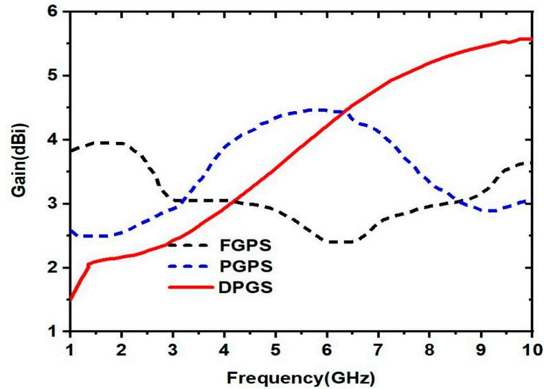
Figure 8. Variations in gain for various ground plane structures.
