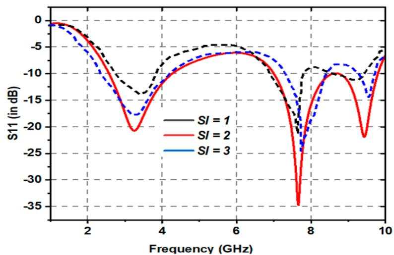
Figure 12. Simulated analysis of  $S_{11}$  (dB) response as a function of  $S_l$ .
