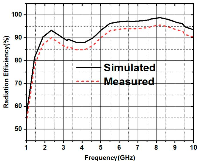
Figure 20. Radiation efficiency plot obtained using both measurement and simulation.
