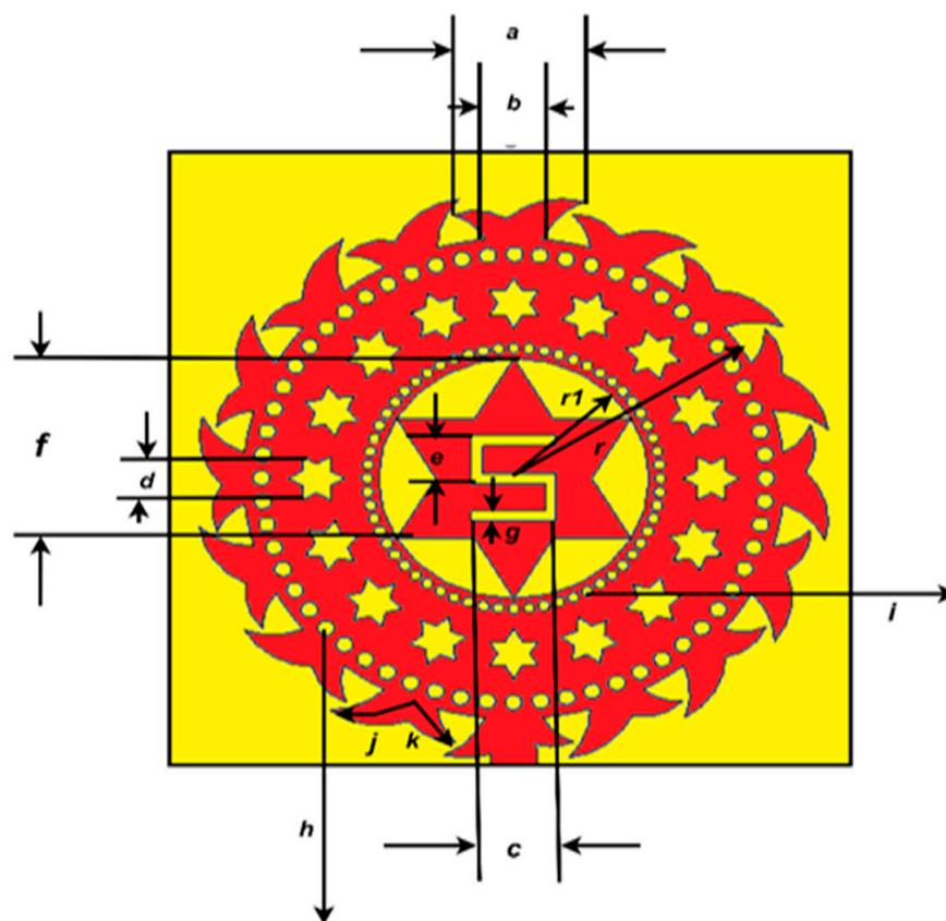
**Figure 3.** Projected view of the radiating patch symbolizing design parameters.
