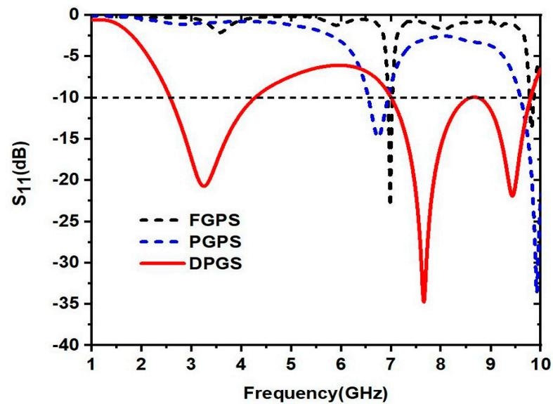
**Figure 7.** Variations in  $S_{11}$  parameters for various ground plane structures.
