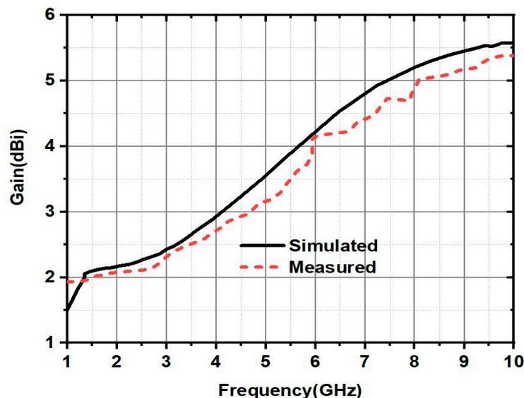
Figure 19. Representation of Gain vs Frequency plot using both measurement and simulation results.
