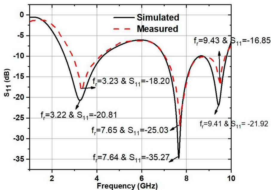
**Figure 16.** Simulated and measured results obtained for  $S_{11}$ .
