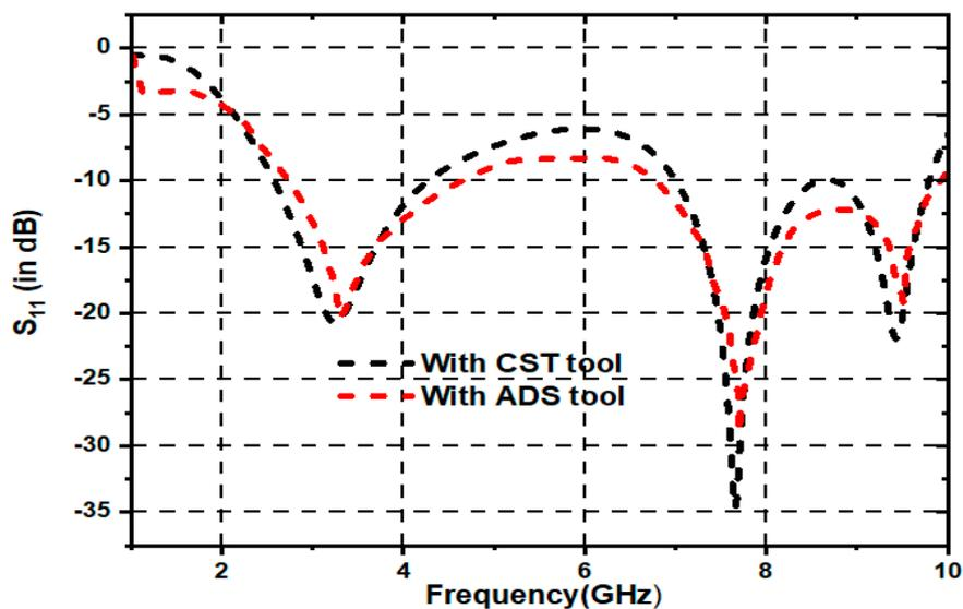
Figure 23. Comparison of the Reflection coefficient in CST and ADS.
