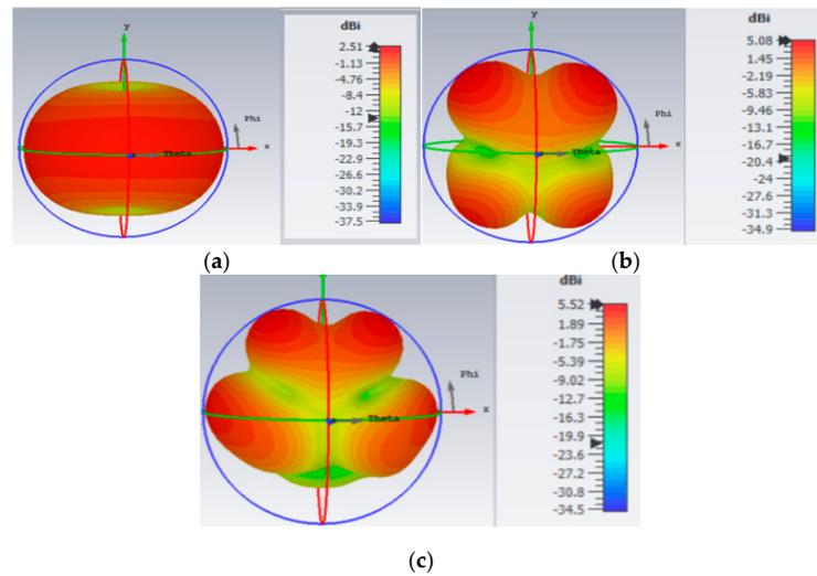
**Figure 17.** Gains at the corresponding resonating frequencies of (a) 3.22 GHz, (b) 7.64 GHz, and (c) 9.41 GHz.
