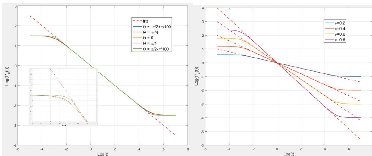
**Figure 6.** Comparison in log–log representation of  $f(t)$  with  $f'_a(t)$  for various values of  $\theta$  and  $\nu = 0.5$  (left) and for various values  $\nu$  and  $\theta = -\pi/3$  (right) for  $t_l = 10^{-3}$ ,  $t_h = 10^5$ ,  $N = 10$ .
