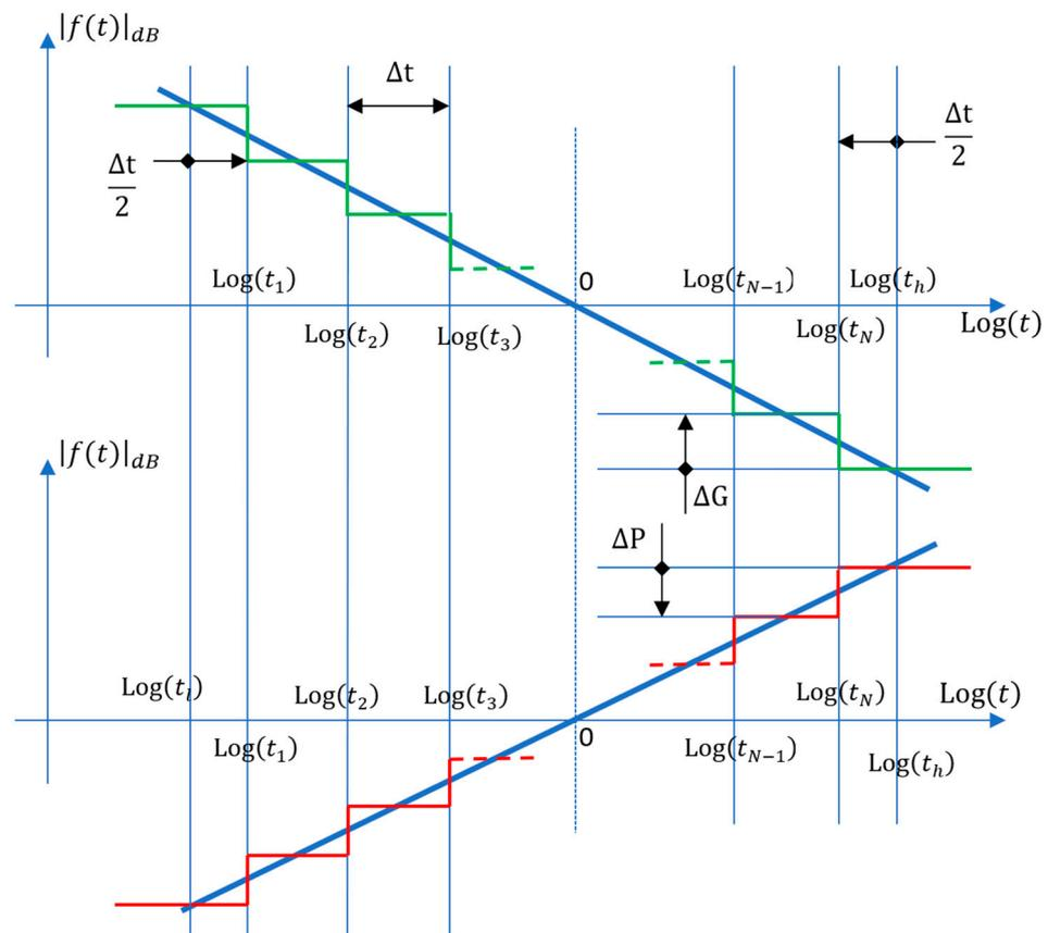
**Figure 9.** Illustration of the gain and phase approximation methodology for  $t^{-\nu}$ ,  $\nu \in \mathbb{R}$ , in log–log representation. Green lines and red lines show the successive asymptotic contributions of poles and zeros to the gain and phase.
