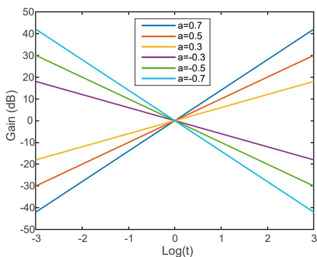
**Figure 7.** Gain of  $f(t)$  (that does not depend on parameter  $b$ ) in log–log representation as a function of  $\text{Log}(t)$  for various values of parameter  $a$ .
