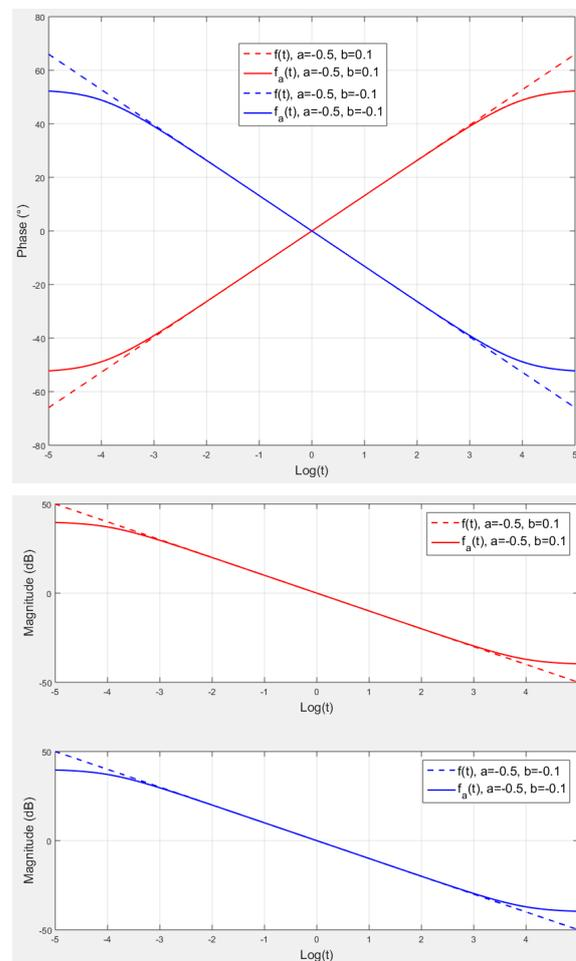
**Figure 11.** Comparison of the gains (top) and phases (bottom) of  $f(t)$  and of its approximation  $f_a(t)$  for various values of parameters  $a$  and  $b$ .
