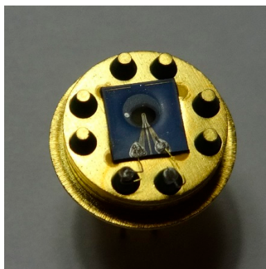
Figure 3. LTCC MEMS with 20 \mu\text{m} thick cantilever laser shaped microheater.
