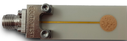
Figure 2. Final sensor device for measuring the reflection parameter S_{11} .
