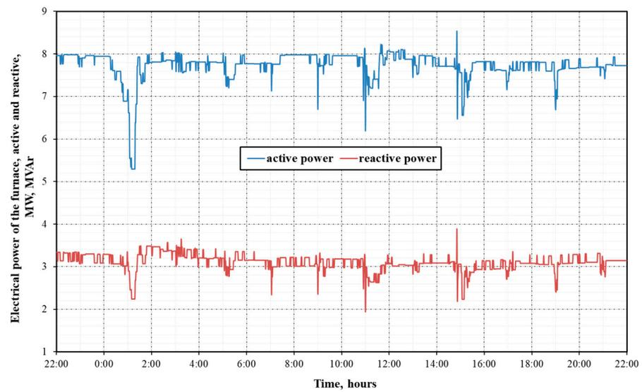
Figure 1. Stream of electric energy supplied to furnace.
