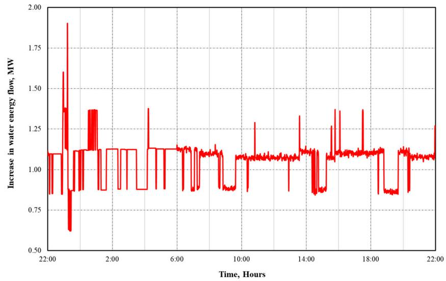
Figure 5. Increase in water stream energy in furnace cooling system.
