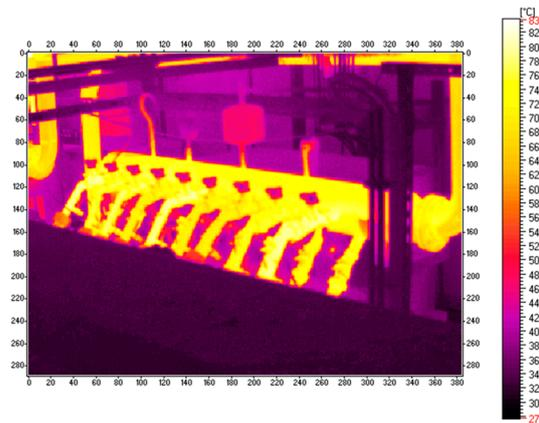
Figure 3. Temperature distribution in the collective collectors of the furnace cooling system.
