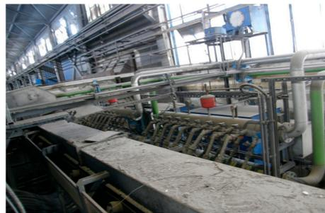
Figure 2. Collective collectors together with elastic pipes of cooling system.
