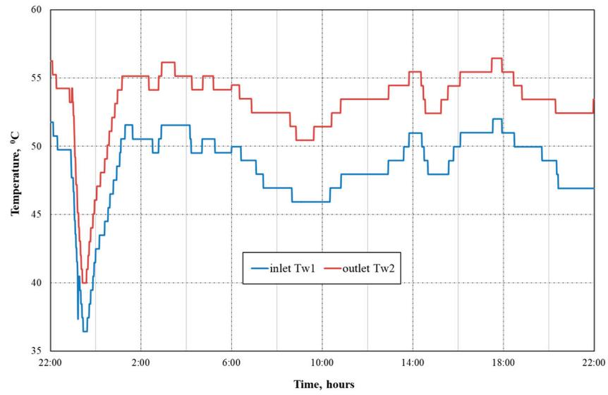
Figure 4. Water temperature in the furnace cooling system.
