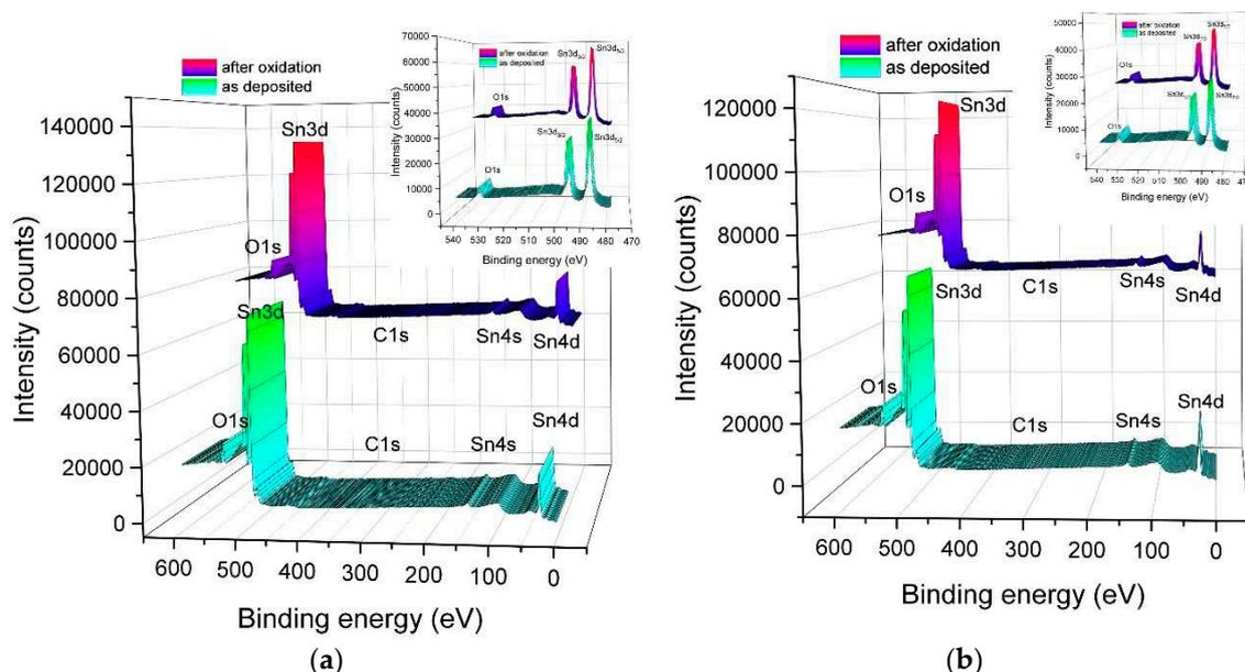
**Figure 1.** XPS survey spectra with the main core level lines of: (a) RGVO SnO<sub>2</sub> nanolayers deposited on SiO<sub>2</sub> substrate both as deposited and after additional oxidation, together with the corresponding O–Sn3d spectral window (in the inset); (b) RGVO SnO<sub>2</sub> nanolayers deposited on SiO<sub>2</sub> substrate modified with Cr and Al additives both as deposited and after additional oxidation, together with the corresponding O–Sn3d spectral window (in the inset).
