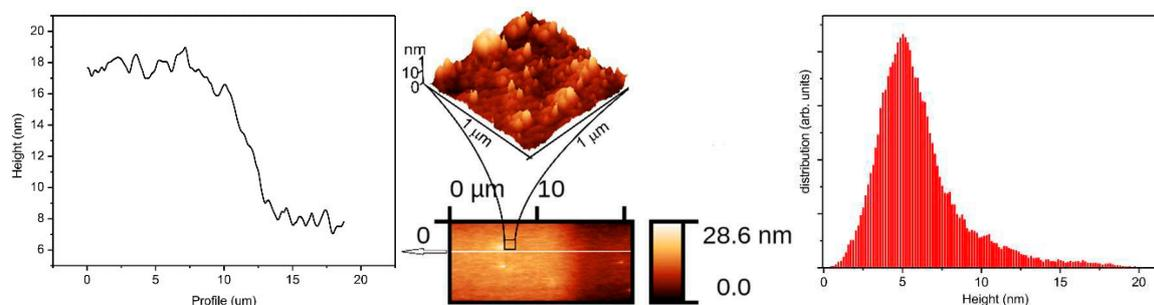
**Figure 2.** AFM data of RGVO SnO<sub>2</sub> nanolayers including the main image, average height distribution and the layer’s edge profile.
