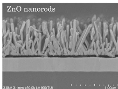
**Figure 1.** SEM image of ZnO nanorods deposited on an ITO substrate.
