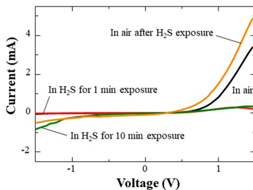
Figure 3. IV curves of the CuO NCs/ZnO NRs device in air and air containing 8 ppm H<sub>2</sub>S at 150 °C.
