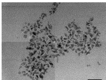
**Figure 2.** TEM image of CuO nanocrystals synthesized by a hot-soap method. The scale bar is 50 nm.
