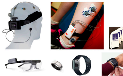
Figure 4. Top from the left: B-Alert X10, Shimmer 3 ECG/EMG/GSR and WideFind UWB-positioning tags. Bottom from the left: Tobii Glasses 2, Oura ring, Empatica E4 and Apple Watch with AliveCor KardiaBand.
