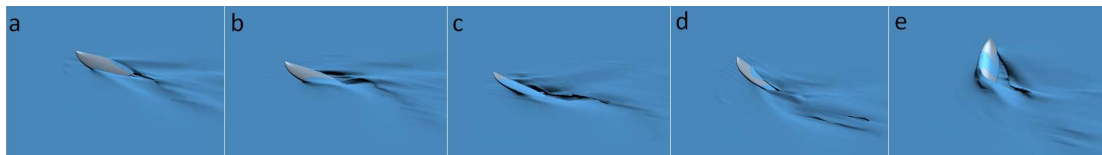
Figure 4. Snapshots of the free surface behind the board at different moments in the maneuvering simulation.
