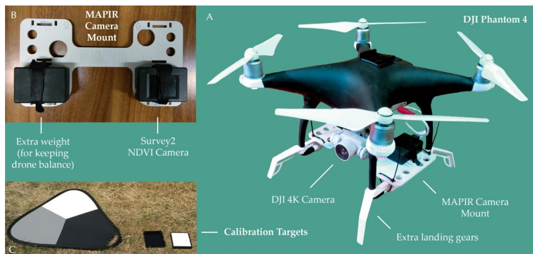
Figure 2. UAV platform: (a) modified quadcopter DJI Phantom 4; (b) Camera mount with Survey2 NDVI Camera; (c) Calibration targets.
