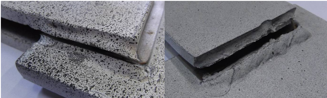
Figure 2. Typical failure mode for longitudinal welds (left) and transverse welds (right).
