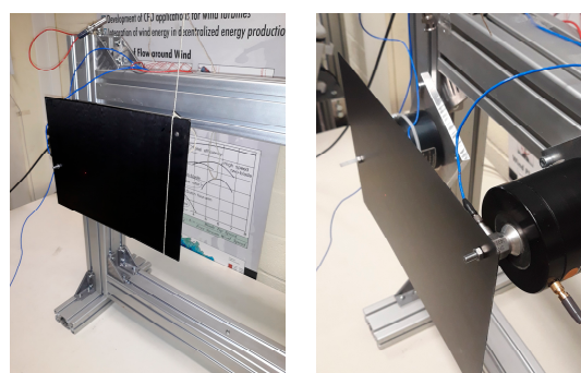
Figure 3. Two different boundary condition scenarios: the plate is fixed on one side and free suspended on the other side (i.e., a free-attached boundary condition) (left); the plate is fixed to two shakers (right).
