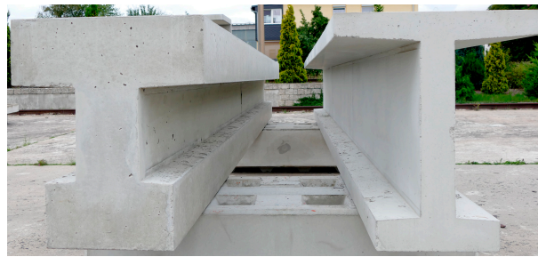
Figure 3. Comparison between (left) a RC and (right) a TRC beam (photo: A. Schumann).
