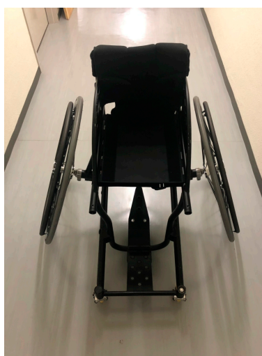
Figure 2. Wheelchair made of magnesium alloy.
