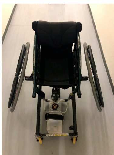
Figure 1. Wheelchair made of aluminum alloy.
