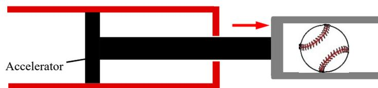
**Figure 2.** Setup of the pitch machine to project baseballs with desired spin rate and spin axis.
