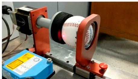
**Figure 4.** Laser profiler used to measure seam height of baseballs.
