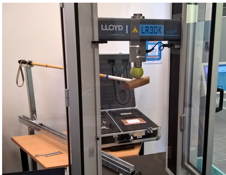
Figure 4. The testing kit with the stick mounted to undertake direct loading in the vertical plane.
