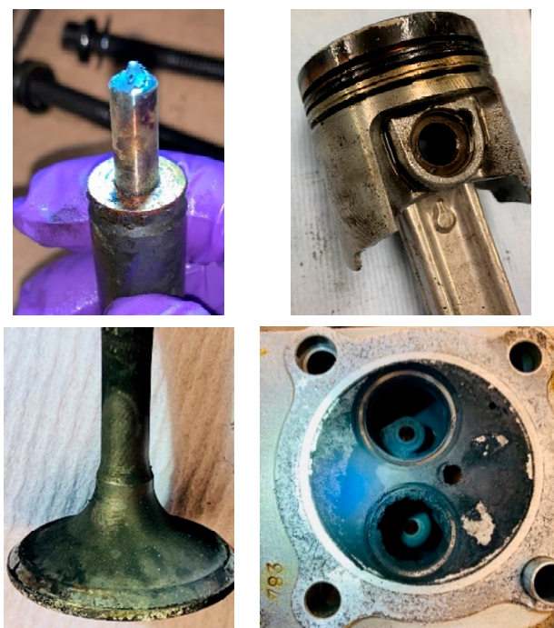
Figure 9. Deposit formation on engine parts.
