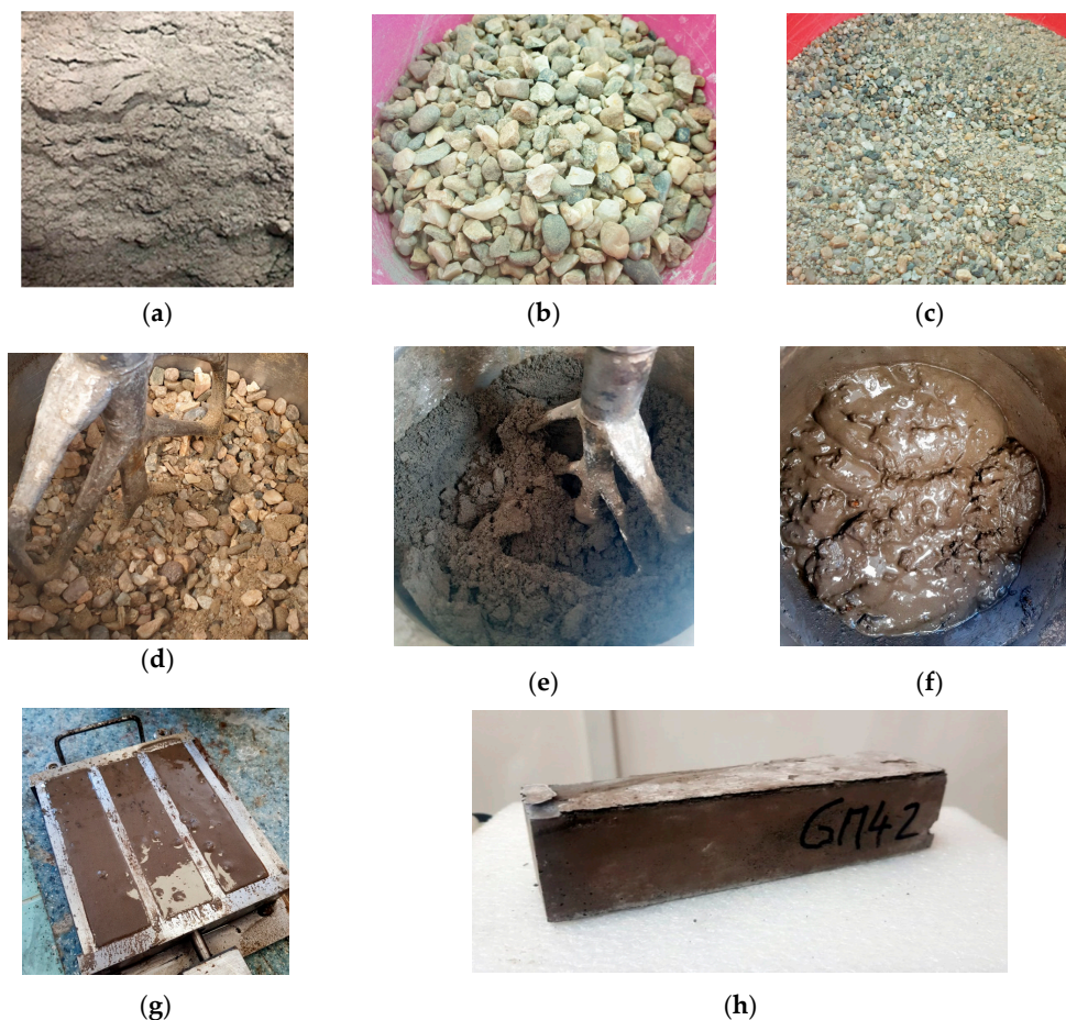
Figure 1. Alkali-activated fly ash-based geopolymer concrete: (a) Fly ash; (b) Coarse aggregate–granular class 4/8 mm (CA); (c) Sand–granular class 0/4 mm (S); (d) Mixing of the aggregates; (e) Mixing of the raw materials (FA + aggregates); (f) Final mixing sequence; (g) Casting of the mixtures; (h) Geopolymer concrete samples after demolding.
