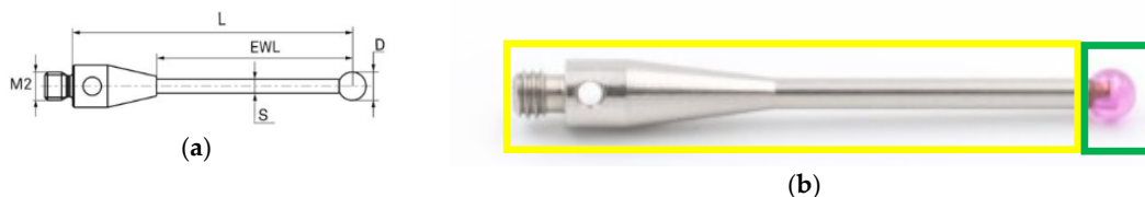
Figure 2. Probe configuration and dimensions: (a) Probe characteristics; (b) Characteristic marked with yellow are inactive and with green are active. “Pitch diameter measurements of internal threads are more complicated than external threads [2] due to construction of internal thread which does not allow easy probing like external threads”.
