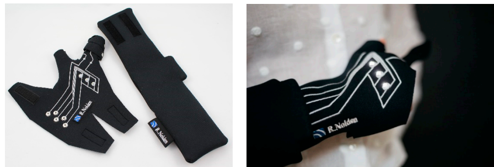
Figure 3. Smart glove and cuff; when forming a wrist, the LEDs light up giving feedback on the intensity of the bending of single fingers.
