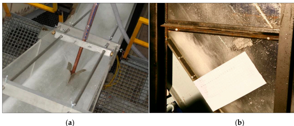
Figure 5. (a) Pitot probe during the velocity measurement process. (b) ACM during the concentration measurement process.
