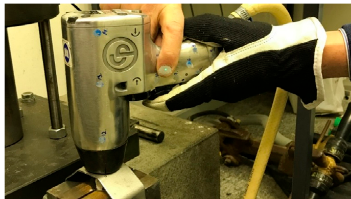
Figure 2. Setup for measurements on the fingernail in position 9. The green dot on the fingernail is the pilot laser that shows where the IR laser measures the velocity.
