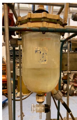
Figure 1. The 20 L reactor used for the synthesis.
