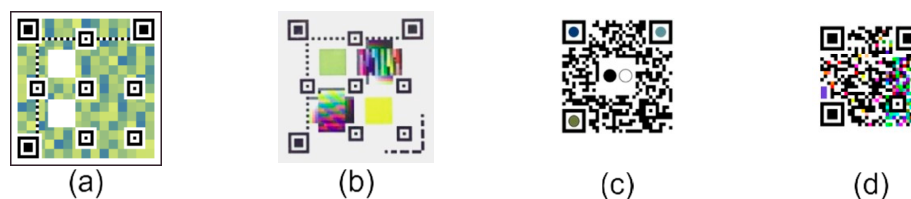
Figure 1. Evolution over the years of machine-readable patterns which embed colorimetric dyes from 2018 to 2023. (a) Our first proposal for such patterns, presented at Eurosensors in 2018 [1]; (b) our second attempt to fabricate the patterns [2]; (c) Escobedo et al. proposal [3] to embed sensors in pattern with digital data; and (d) our proposal to do a similar concept but maximizing back-compatibility [4].
