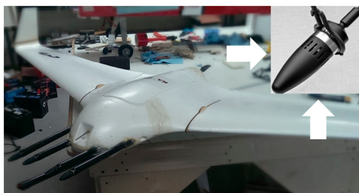
Figure 3. Delta X-8 fitted with four DPA 4053 microphones with a close-up of the sensor in the top right sub image.
