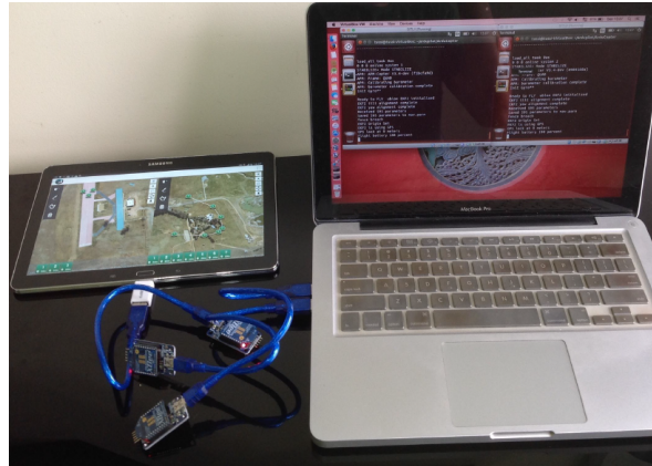
Figure 3. Experimental Setup: Ground Control Station running on the Android Tablet; two instances of drones running in the STIL in the notebook; and the XBee modules used as communication devices.
