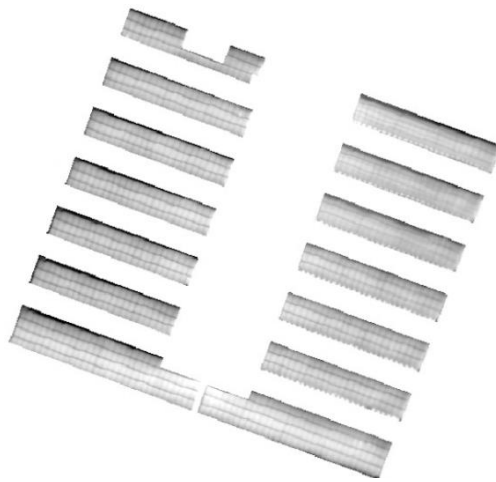
Figure 23. Extracted modules on thermal orthomosaic.
