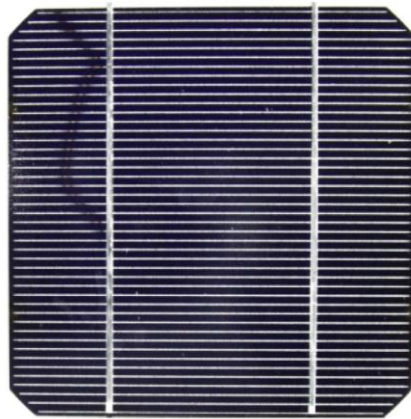
Figure 6. Phenomenon of snail trails in a PV cell [8].
