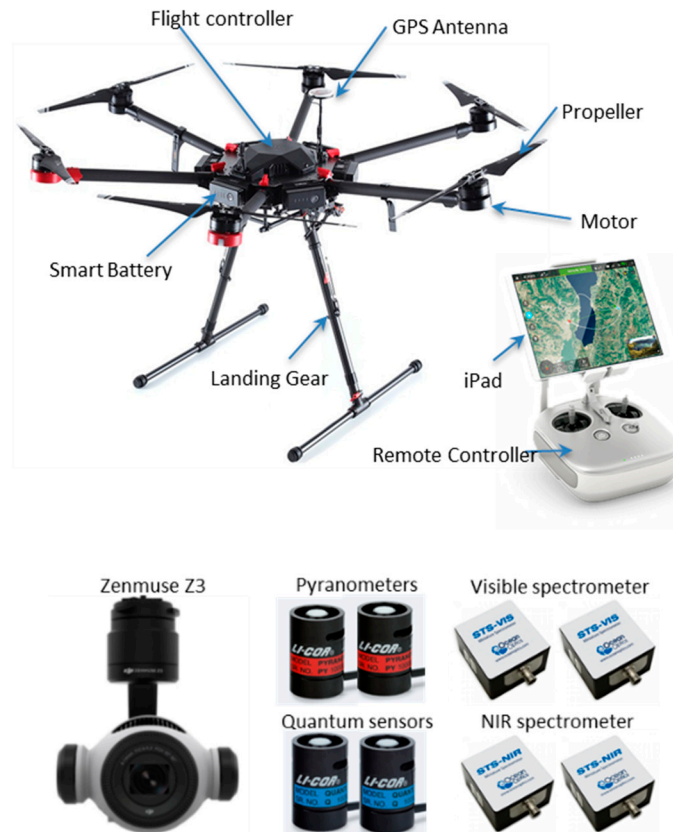
Figure 1. The Matrice 600 UAV, Zenmuse Z3 camera, pyranometers, Quantum sensors, and Visible and NIR spectrometers.
