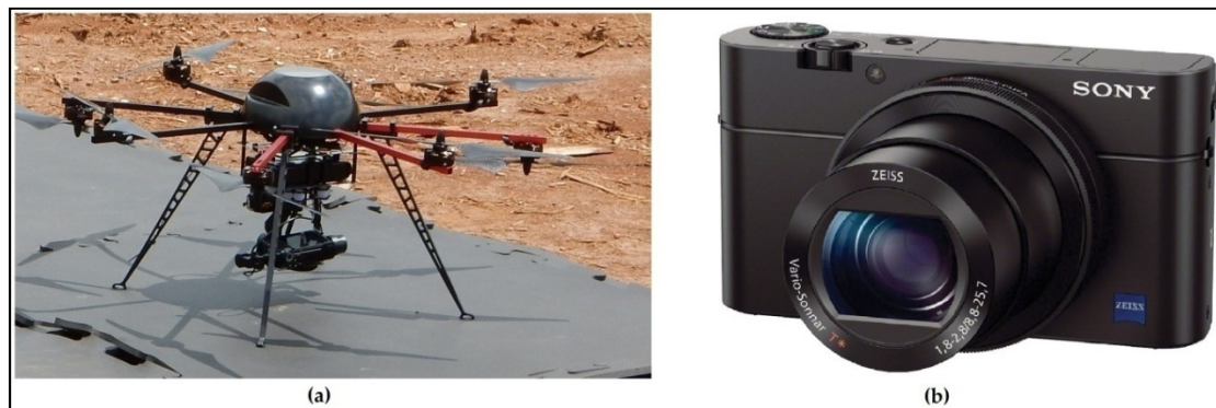
Figure 2. (a) Octocopter GYRO 200 OCTA 355 UAV; (b) Sony RX100M3 camera of 20.1 megapixels.
