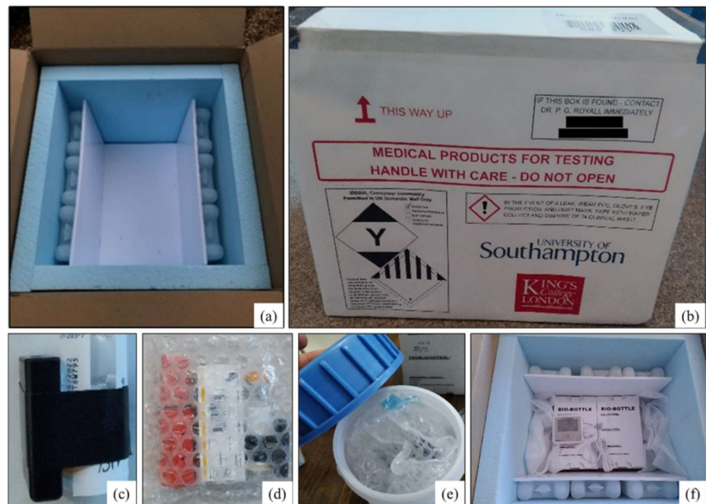
Figure 6. Insulated polystyrene and cardboard based packaging. Chilled with cooling packs shown. Approximate dimensions 32 cm × 37 cm × 36 cm, empty weight inc. cool packs ~6 kg. (a) internal, (b) external. (c–f) packaging configuration: (c) insulin vial with attached vibration sensor, (d) bubble wrap bag with monitored vial and vial box (containing vibration sensor) and temperature sensor, (e) blue bio-bottle containing wrap bag with vials, (f) cooled cytotoxic drug box containing two boxed bio-bottles and MHRA certified temperature sensor.
